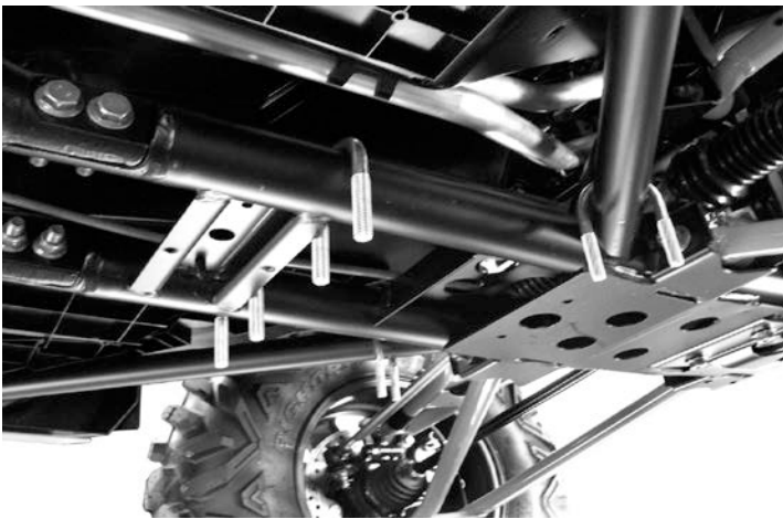
U-bolt placement on the frame tubes.
