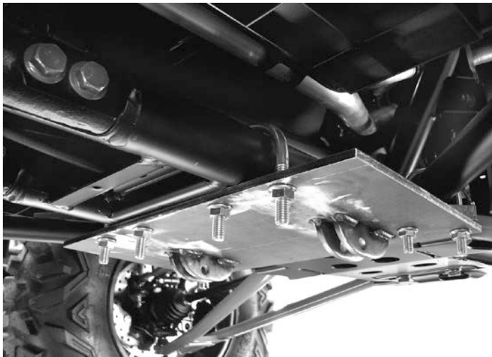
Place the over the u-bolts and secure with washers and nylock nuts.
